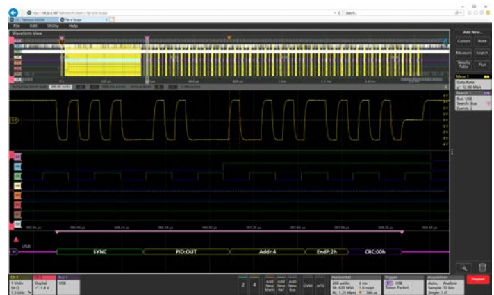
Figure 34: e*Scope provides simple remote viewing and control using common web browsers.
