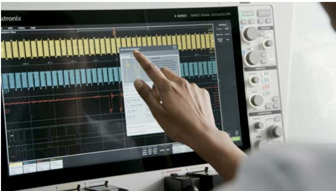
Figure 8: Interact with the capacitive touch display in the same way you do on your phones and tablets.
