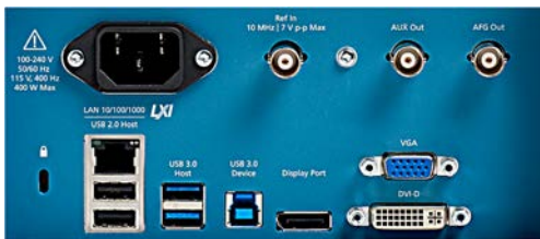
Figure 33: The I/O you need to connect the 6 Series MSO to the rest of your design environment.
