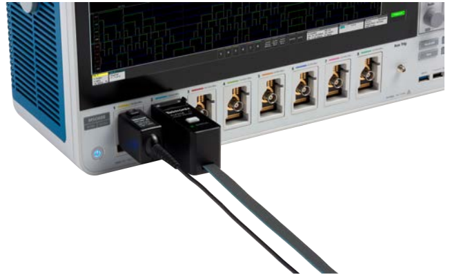
Figure 1: FlexChannel technology enables the ultimate in flexibility. Each input can be configured as a single analog or eight digital channels based on the type of probe you attach.
