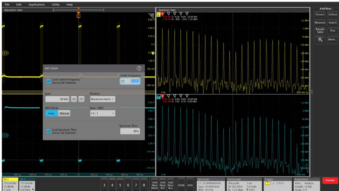
Figure 25: Intuitive spectrum analyzer controls like center frequency, span and resolution bandwidth (RBW), independent from time domain controls, provide easy setup for frequency domain analysis. A spectrum view is available for each FlexChannel analog input, enabling multi-channel mixed domain analysis.
