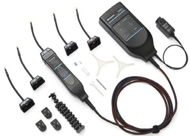
Figure 19: The Tektronix TIVM Series IsoVu™ Measurement System offers a galvanically isolated measurement solution to accurately resolve high bandwidth, differential signals up to 2,500 Vpk in the presence of large common mode voltages, with the best in class common mode rejection performance across its bandwidth.
